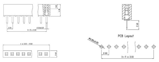
When using the recommended connector, ensure that any baseboard components placed under the Skywire (between the baseboard header pin connectors) are no taller than 4 mm. However, please note that the maximum component height may change based on the chosen baseboard connector.
