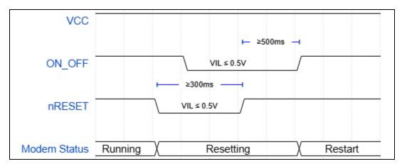
It is necessary that this signal be connected to the host system. It should be driven with an open collector output from the host system or a discrete open collector transistor. To avoid damaging the modem, this signal must never be driven high with a push-pull I/O pin.
